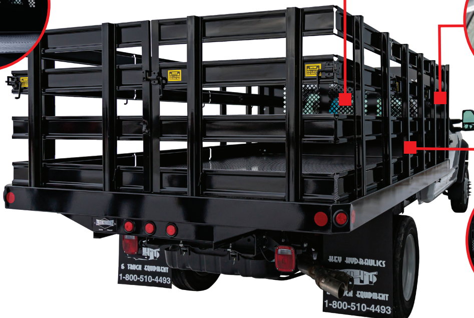
SPRING-LOADED, EASY-TO-ATTACH FRONT RACK LOCKS
